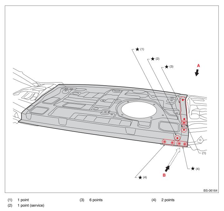
For locations marked by "★": the welding method and the number of welding points are the same on the left and the right.
